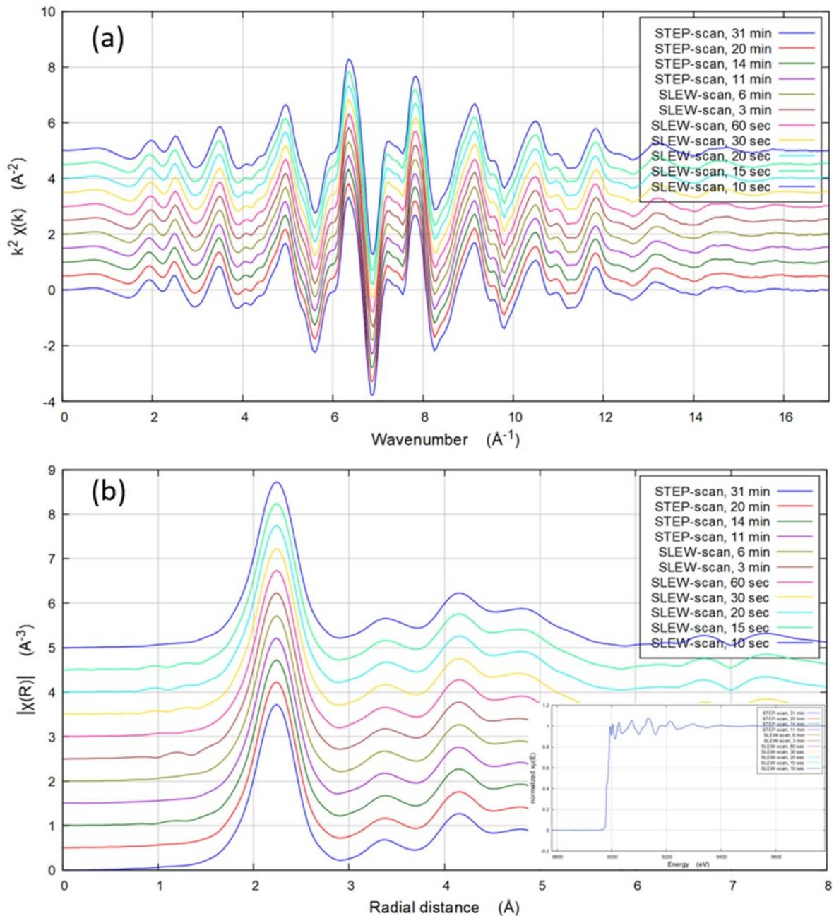
Fig. 1: XAS spectra for bulk metallic Cu measured both using step-scan (31, 20, 14, and 11 minutes) and using slew-scan (6, and 3 minutes, and 60, 30, 20, 15, and 10 seconds), with (a) the post-edge XAS region, and (b) the corresponding Fourier-transformed signal. The inset shows the 11 scans overlaid in energy space
