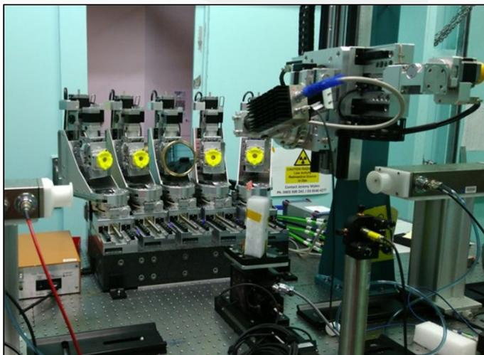
Fig. 1: (Top) Schematic of crystal spectrometer and (bottom) photo of the MEX crystal spectrometer, currently hosted at the XAS beamline, Hutch C.
