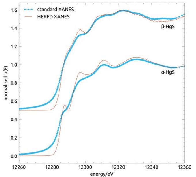
Fig. 2. Preliminary data from the spectrometer in comparison to standard XANES of the mercury edge, on samples containing approximately 2000 ppm Hg. The  $\beta$ -HgS scan was a single XANES scan collected over 30 min, while the  $\alpha$ -HgS is an average of five 30 min scans
