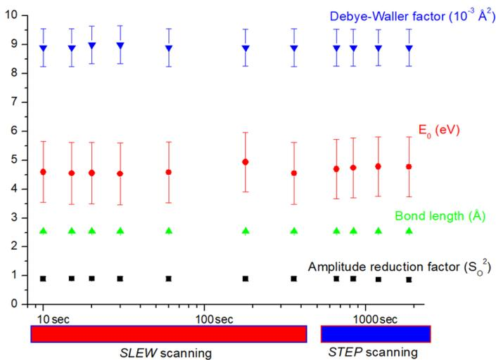
Fig. 2: XAS data parameters extracted from the scans shown in Figure 1 and plotted as a function of scan time. Special thanks to Simon James, MEX Beamline, for doing the data analysis
