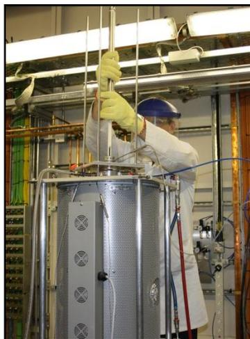
Experimentalist loading an electrode stalk into the furnace.
