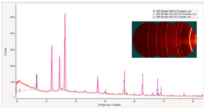
Figure 3. Phase identification was undertaken on sample C1 using the refined search criteria based on the Tornado  $\mu$ -XRF findings. Inset shows the combined 2D detector images for this sample.
