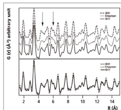
Figure 3. Comparison of the PDF obtained with data from the beam lines and the Empyrean diffractometer [2].
