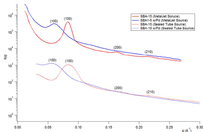
Figure 1. Scattering curves from the new MetalJet-D2 X-ray source (solid line) and the previous Cu sealed tube (dotted lines). The curves were corrected for collection time and the use of an Al foil to attenuate the beam from the MetalJet-D2 source (to prevent saturation of the detector). The curves are of samples of SBA-15 (red) and SBA-15 that has been doped with palladium nanoparticles (blue).
