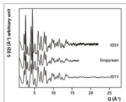
Figure 2. Structure function  $S(Q)$  comparison between two synchrotron beam lines and the Empyrean with GaliPIX<sup>3D</sup> [2].
