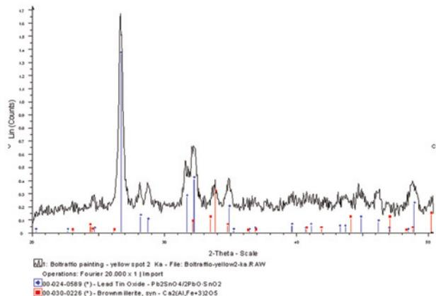
Figure 2. XRD data collected on Boltraffio's yellow – 50 min integration.
