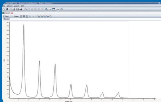
Figure 2: Low angle data collected on silver behenate. Thanks to the Motorized Anti-Scatter Screen and the Variable Active Detector Window™ of the LYNXEYE XE-T the instrument background is extremely low.
