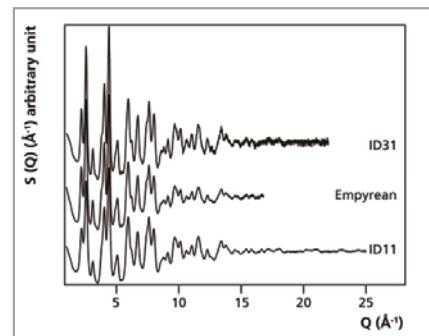
Figure 2. Structure function  $S(Q)$  comparison between two synchrotron beam lines and the Empyrean with GaliPIX<sup>3D</sup> [2].
