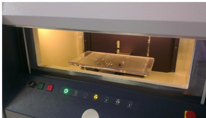
Figure 2. Samples mounted in the 30 well plate being loaded into the Tornado  $\mu$ -XRF for rapid chemical analysis.
