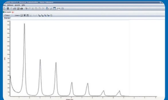
Figure 2: Low angle data collected on silver behenate. Thanks to the Motorized Anti-Scatter Screen and the Variable Active Detector Window™ of the LYNXEYE XE-T the instrument background is extremely low.
