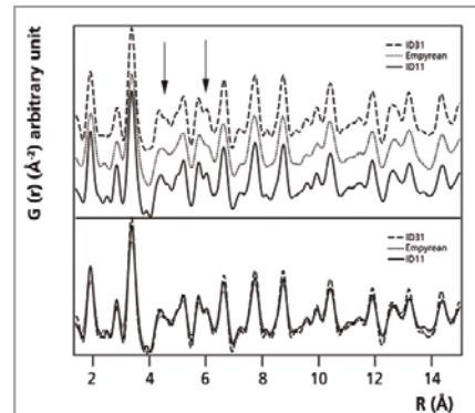
Figure 3. Comparison of the PDF obtained with data from the beam lines and the Empyrean diffractometer [2].
