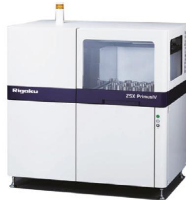
The new Rigaku Primus IV WDXRF spectrometer.
