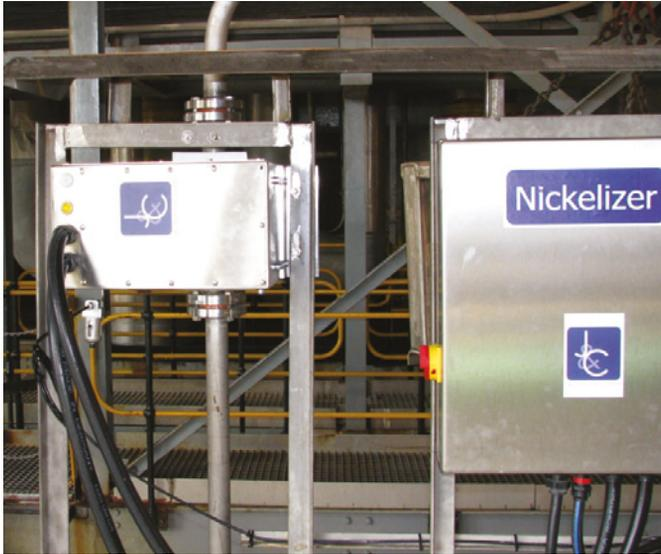
IMP's Online Pipe XRF Analysis System is an online X-ray fluorescence device for the elemental analysis of slurries or suspensions without sampling.
