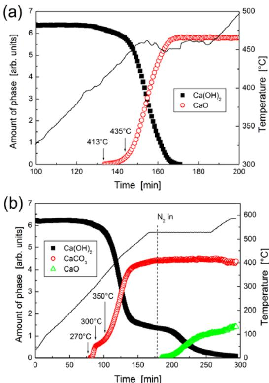
Figure 1. Phase transformations of crystalline species during the (a) dehydration in N<sub>2</sub> and (b) superheating in CO<sub>2</sub>, of Ca(OH)<sub>2</sub>. Reproduced from Materić, Ingham, Holt; *CrystEngComm* 2015, 17, 7306.
