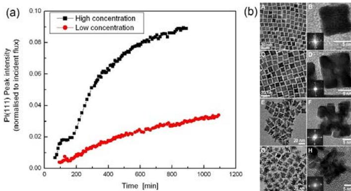
Figure 2. (a) X-ray diffraction intensities of Pt nanoparticles during formation. The high concentration experiment shows multiple stages, illustrated by transmission electron microscopy images in (b), recorded after (A, B) 75 min, (C, D) 120 min, (E, F) 240 min, (G, H) 500 min. Adapted from Cheong, Watt, Ingham, Toney, Tilley; *J. Am. Chem. Soc.* 2009, 131, 14590.
