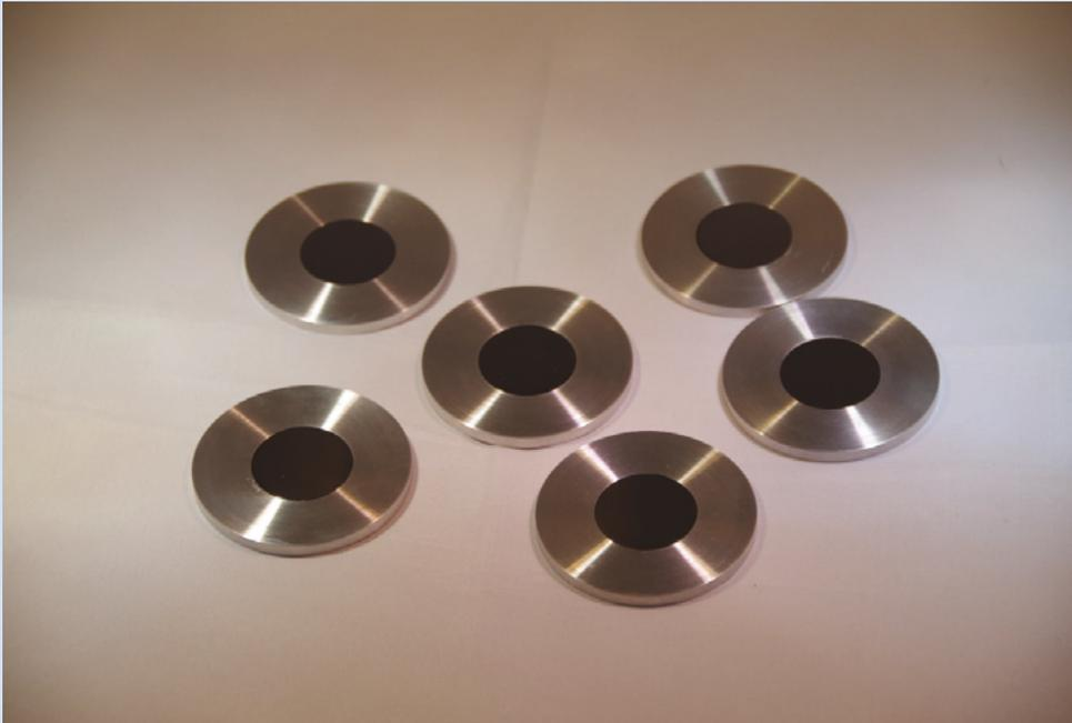
The photograph shows sample holders fitted with Silicon inserts. The surface is set 0.1 mm below the surface of the sample holder. We can modify your existing holders or make new holders to match your existing holders.
