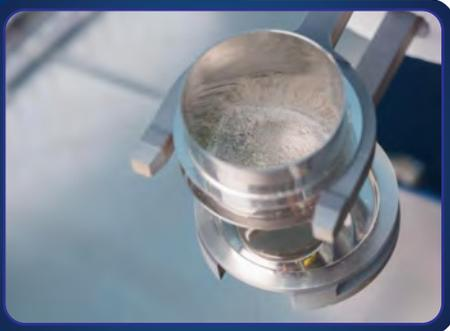
The Bead One R is able to perform different sample preparation processes in an inert gas or oxygen atmosphere.
