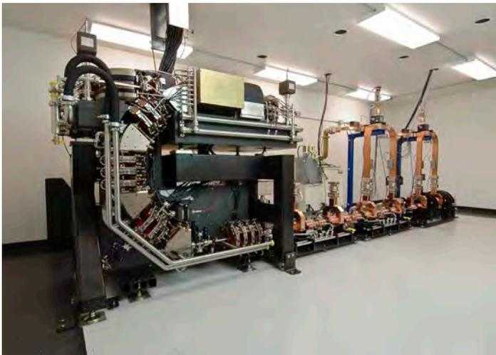
**The Lyncean Compact Light Source, a laboratory based, mini-synchrotron for production of high brilliance radiation.**
