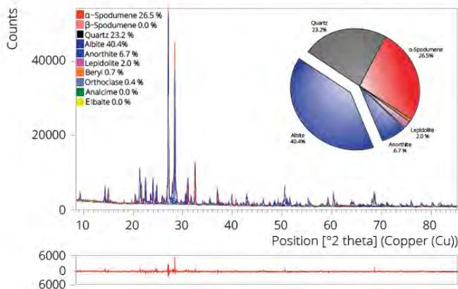
Figure 2. Quantitative Rietveld analysis of a complex lithium ore
