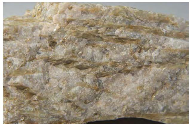
Figure 1. Hard-rock lithium ore
