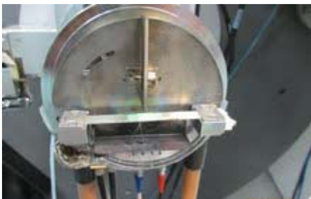
Sample mounted on platinum strip in furnace for in-situ HT-XRD experiments.
