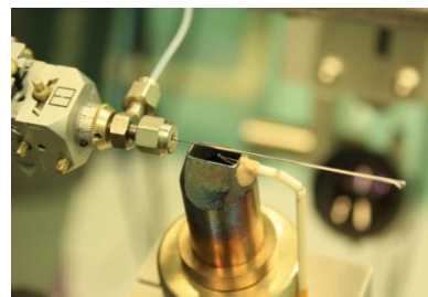
Left) Overview of the basic Norby cell design [1]. Above) Photograph of a Norby cell being used during a high temperature oxidation study at the Australian Synchrotron. The cell is being heated by the hot-air blower shown at the bottom of the photo.
