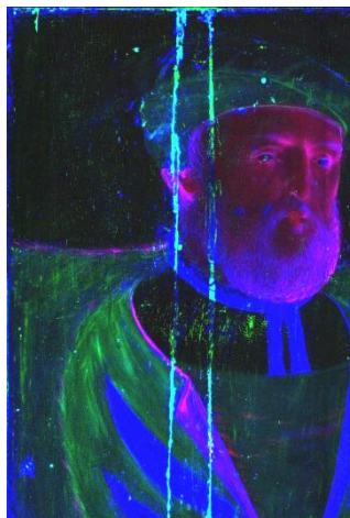
(Left) RGB composite image of Henry VIII portrait showing mercury (red), calcium (green), and iron (blue) collected on the prototype milliprobe. (Right) Mockup of milliprobe large area (0.6 m X 1.2 m) scanning stages with \sim 50 \mu\text{m} resolution.
