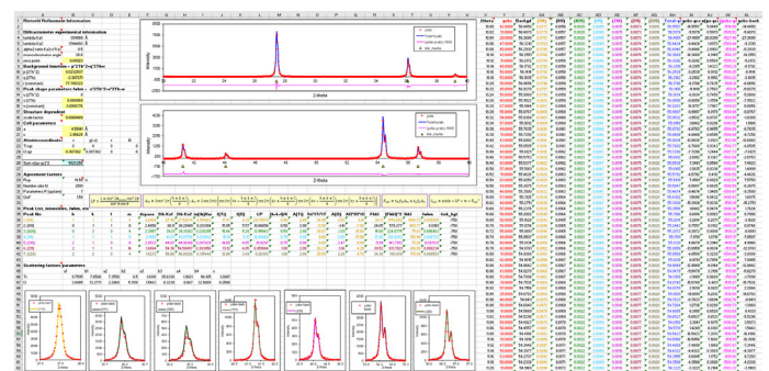
Figure 1. The teaching tools developed by Evans and Evans begins with a simple least-squares fit (top) and expands to a full Rietveld refinement (bottom).
